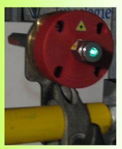
THE SLM-515S AND SLM-635S MOUNTING AND ADJUSTMENT SYSTEM is manufactured using FRAS approved materials and precision adjustment mechanisms. The two adjustment knobs provide adjustment in horizontal and vertical directions about a fixed pivot. The adjustment system is spring loaded to maintain pressure on the adjustment feet, while the fine adjustment threads allow for precise adjustment even over long distances.
