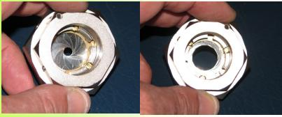
Adjustable IRIS system to aperture the beam down to 1mm for close-up, precise alignment.
