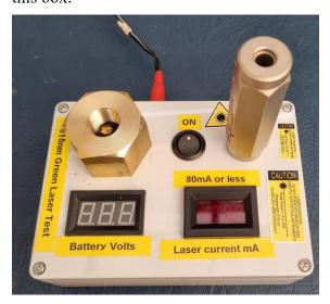
Switch the ON switch to power up the laser, BEING AWARE THAT THE LASER WILL EMIT UPWARDS. ENSURE THAT YOU ARE NOT LOOKING INTO THE LASER!!! The laser current will be displayed. If the laser current is > 80mA or approaching 80mA, then the laser will blow battery module fuses and needs to be serviced with a new laser module. Laser currents can vary quite a bit, anything under 70mA is still good.
