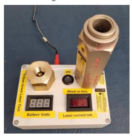
Turn on the 7.5V supply with the switch and test the laser head. Return to ART for service is approaching or exceeding 80mA.
